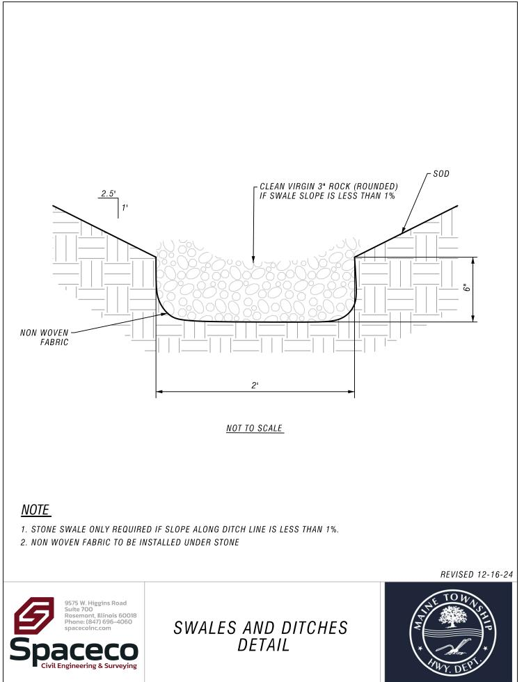
N:\Projects\6421\6421 Projects\6421.97 - Engineering Standards\NEW DETAILS\New Maine Township Details\_OSD.dgn 20- SWALES AND DITCHES DETAIL User=srot
